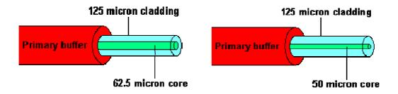
The photos above illustrate that the outer diameters of the two fiber types are the same. What is different is the size of the center light carrying core of the fiber.
